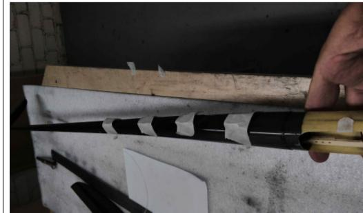
To install the guide tubes, use a long straight piece of music wire, about 0.8mm in diameter. Insert the wire into the tube, position it inside the fuselage, and use small magnets to hold the wire with the tube in place.
