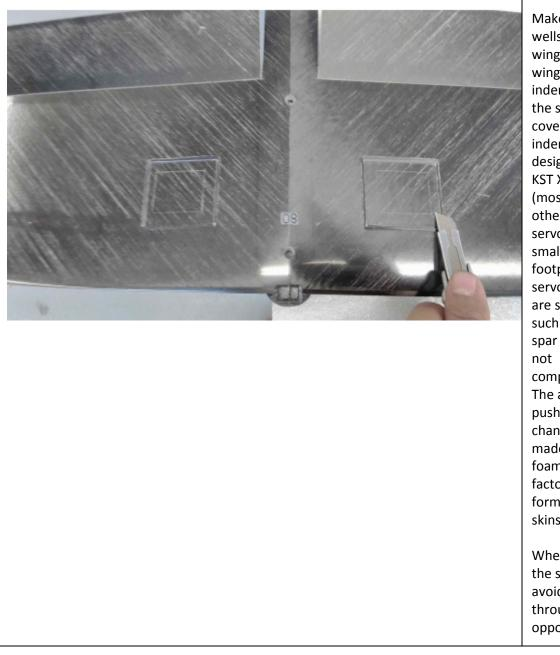
Make servo wells in the wings. The wings have indentations for the servo covers. The indentations are designed for KST X08 servos (most of the other suitable servos have smaller footprint). The servo locations are selected such that the spar strength is compromised. The aileron pushrod channels are made in the foam core at the factory prior to forming the skins.
