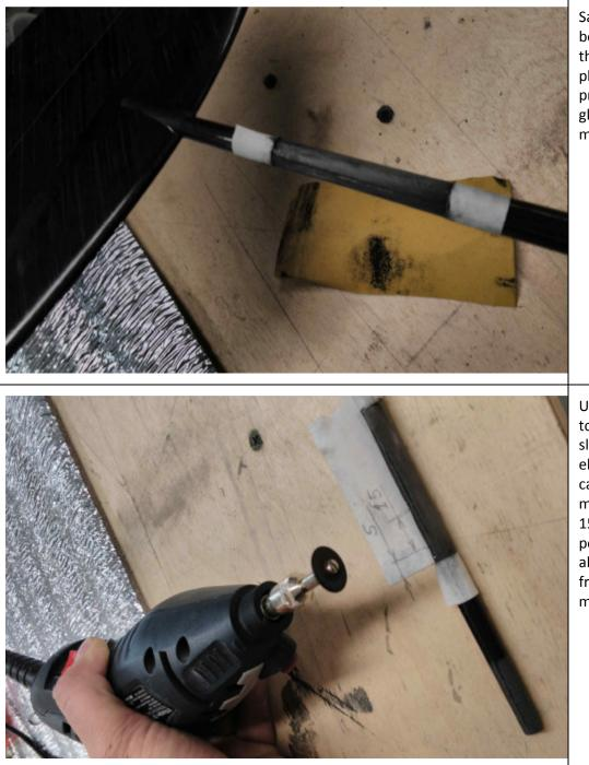
Sand the tail boom between the marked places to prepare it for gluing the stab mount.
