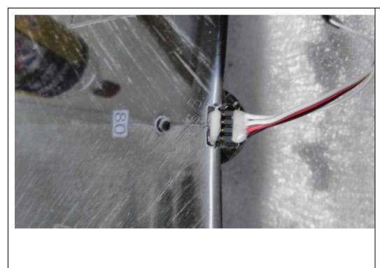
Insert the wing part of the connector into the wing hole. Pull the servo wires from the pockets to remove the slack and allow the connector to sit deep in the hole.
