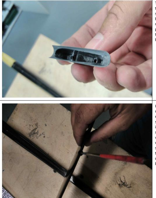
The objective is to remove the shine from the base of the stab mount for proper adhesion to the tail boom.
