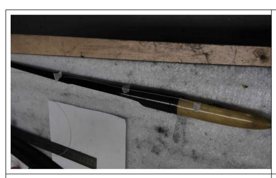
It is recommended to install guide tubes for the control cables, which extend to about the trailing edge of the wing.
