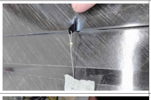
Pull the rudder cable through the tail boom. Attach the rear end to the control horn with a crimp.
