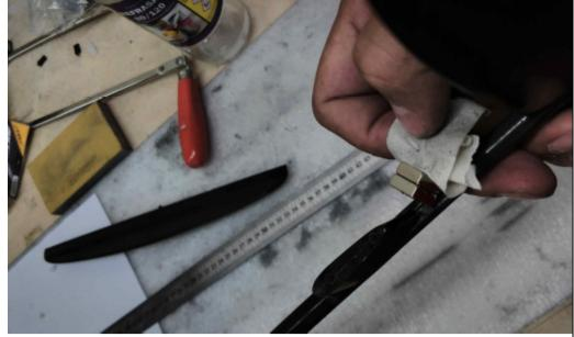
Repeat the procedure with the elevator cable. Guide the wire through the exit hole under the stab mount using a magnet.
